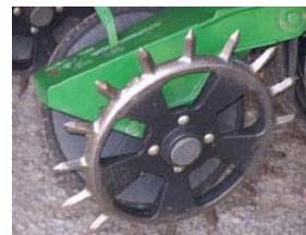
Spiked tooth press wheels for minimum till or no-till conditions.
